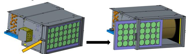
Simply rotate the tabs on each side of the filter frame to access the filter.
